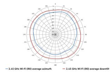
Figure 1. 2.45 GHz Wi-Fi antenna patterns (horizontal)
