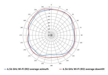
Figure 3. 6.56 GHz Wi-Fi antenna patterns (horizontal)
