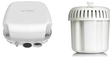
Figure 3. For hazardous location requirements, Aruba provides C1D2 and ATEX Zone 2 certified access points. Lightweight and ruggedly constructed, these access points support IT, IoT and operational technology devices in hazardous locations.
