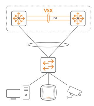
Figure 1: Aruba Virtual Switching Extension
