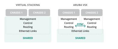
Figure 3: Comparison of Virtual Stacking and VSX
